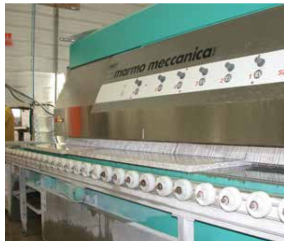
B2B photo by Sean Fitzgerald High-speed water jets polish recently cut decorative stone at AMC of Wisconsin to make smooth countertops.
